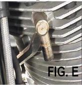
*NOTE:* The air fittings are very tight in the cylinder head. We have found that when driving out the air fittings, the 90-degree joint may start to tear apart. If this happens, simply insert your removal tool into the hole in the
