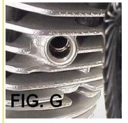
Insert frozen plugs into the vacated fitting holes pushing them in by hand as far as possible. Then using a mallet along with the supplied Baron aluminum drift, gentle drive these plugs into cylinder head/s (FIG. H) below.
